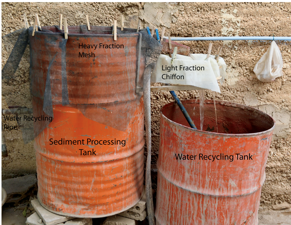
Figure 4. Flotation device with components mentioned in the text labeled. Photo by Martin Weber, 2012.
