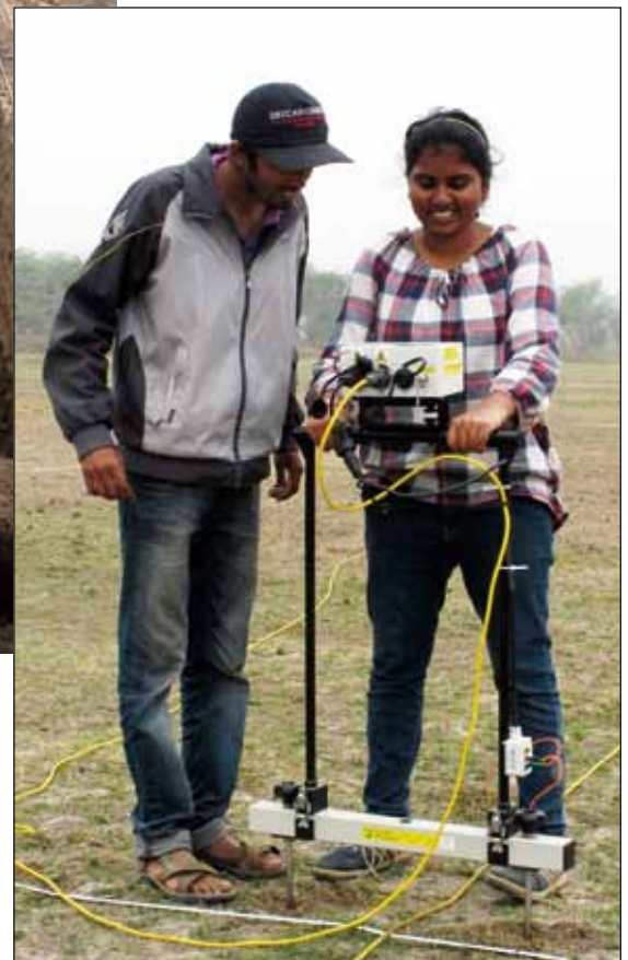
Figure 2. Students with electrical resistivity meter conducting geophysical survey.
