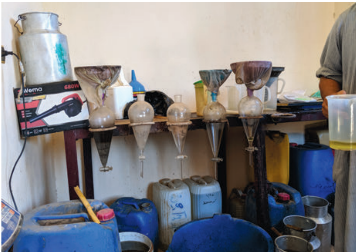
Figure 3. Oil collected from the tanks is filtered with cheesecloth and allowed to separate from any water that remains in glass vials. The water sinks to the bottom tip of these vials and can be drained before the raw oil is collected in large plastic tubs.
