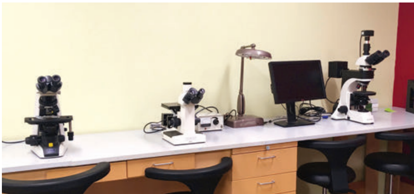
Figure 2. Two polarized light microscopes and a metallographic microscope (center) are available for the examination of samples.
