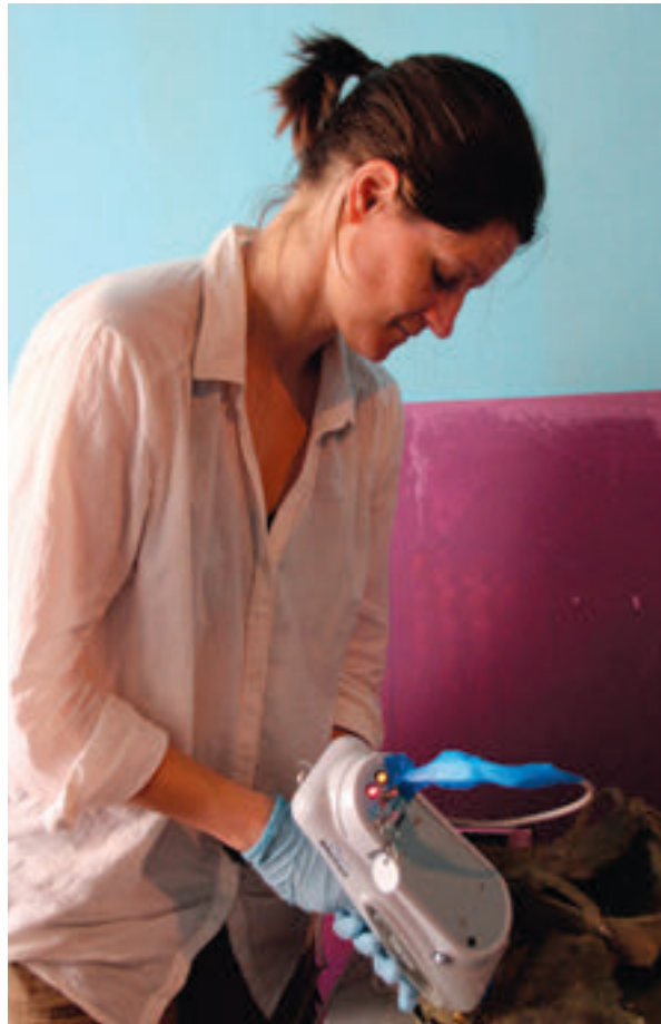
Figure 3. Brittany Dolph Dinneen uses a handheld XRF spectroscopy instrument to investigate the composition of a copper alloy cauldron found by the Naxçivan Archaeological Project, Azerbaijan. (Photograph by Kellen Hope)
