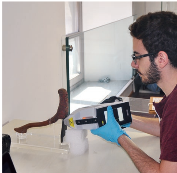
Figure 2. Jeff Newman analyzes the metal blade of an ancient adze with a portable X-ray fluorescence instrument.
