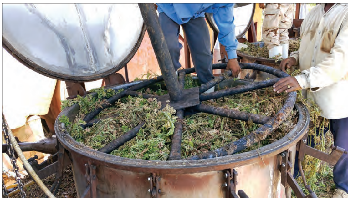
Figure 2. A large metal wheel is inserted both at the bottom and top of a steel tank, and to mash the freshly packed geraniums before steaming. The weight of the wheel, in addition to that of several men standing in the tanks, allows for the processing of large quantities of plant material at once.
